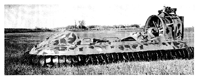
Hovercraft America's vehicle is equipped with a gel-coat hull, 5 passenger (1000 lb) capacity, 130 hp 4-cycle engine, positive air brake system, 84 segement Type-S skirt sytem.
