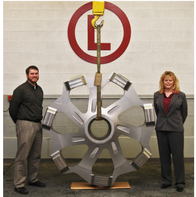
Rotor Hub from a CH53 Heavy Lift Helicopter produced at ATI Ladish Forging
