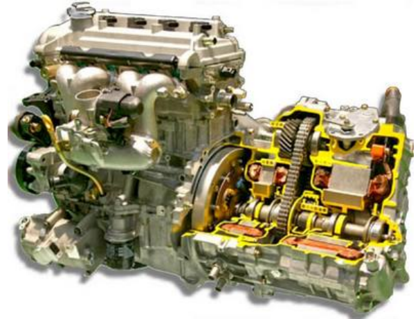
Cut away of Toyota hybrid drive
