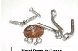
**Metal Parts by Laser Sintering**
