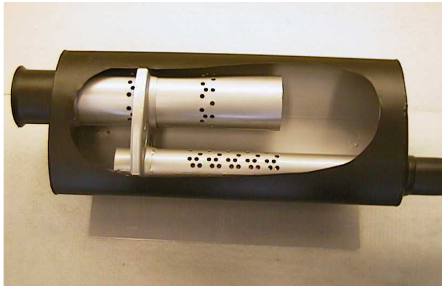
Muffler Cut-Away Example
